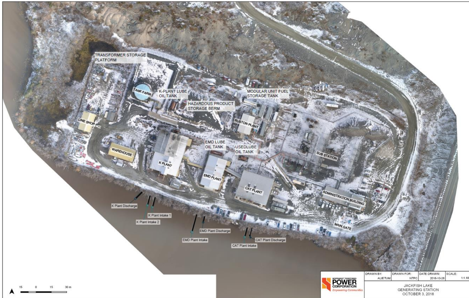
Figure 2-2: Location of Main Hazardous Materials Storage at the Jackfish Facility
