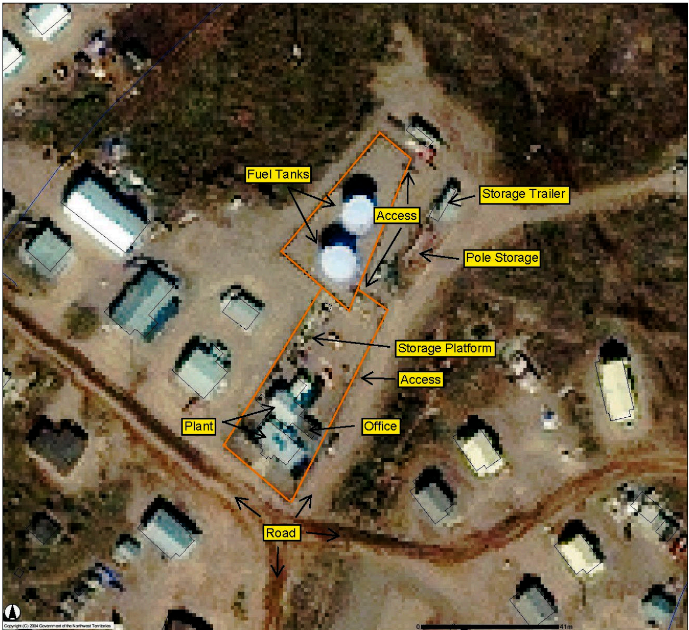
Figure 1: NTPC Plant Site Area – Deline
